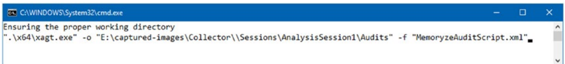
Figure 6-25. CMD window appears while the collector is running; upon finishing, the CMD should disappear without showing any message
