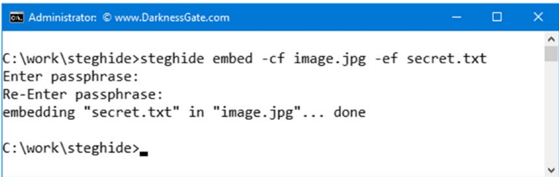
Figure 9-2. Using Steghide tool to conceal a secret text file in an image file
